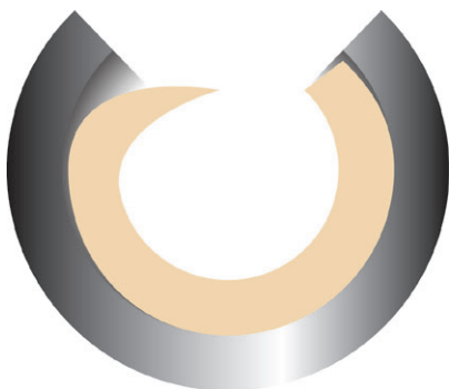
Self-lubricating with teflon liner
