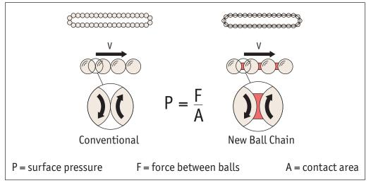
The rotating balls in conventional profile rail quides have point contact between each other. The rotation speed at the contact point is double the speed of the balls. The contact area (A) is so small that the surface pressure (P) tends towards infinity. This leads to heating and wear of the balls and the linear guide system.
