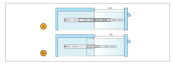
**Full extension** This type of drawer slide can be extended 100% of slide length, this is standard for
